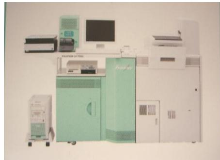
Equipment For Automatically Developing Photographic Paper In Roll
